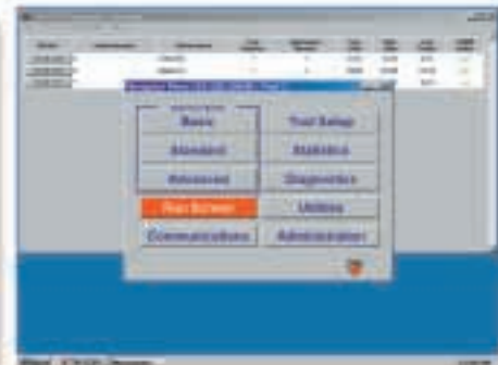
Clicking on an IP address launches a detailed communication session with the TME or TMEM I/O associated with that IP address. The initial screen in this session is the familiar Navigator Screen.
