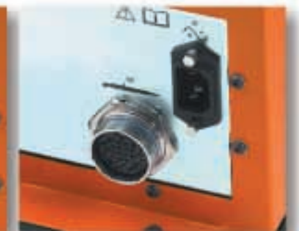
The standard TME is very simple – only 3 connectors – power, tool, and serial for programming.
